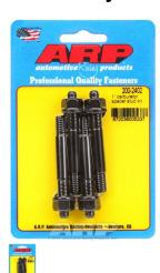
Carburettor Stud Kit, Hex Nut Black Oxide Suit Carburettor With 1" Spacer 5/16" Thread x 2.700" OAL (4-Piece)
